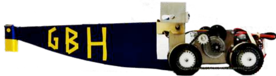
Arm attachment added to knock down the hard teeter-totter obstacle.
