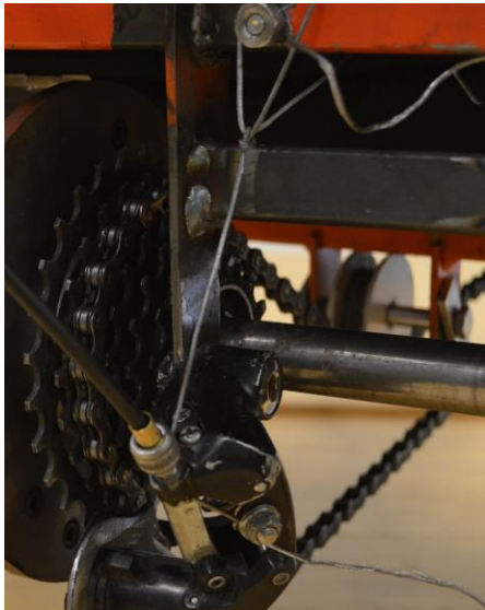
The Arced Slot Used for Adjusting the Derailleur Position at its Highest Position.
