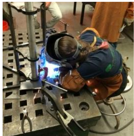
Welding the gusset shaft collar sub-assemblies to the base of the diwheel frame. The vertical aluminum shaft was used as a jig for rigid alignment during welding.
