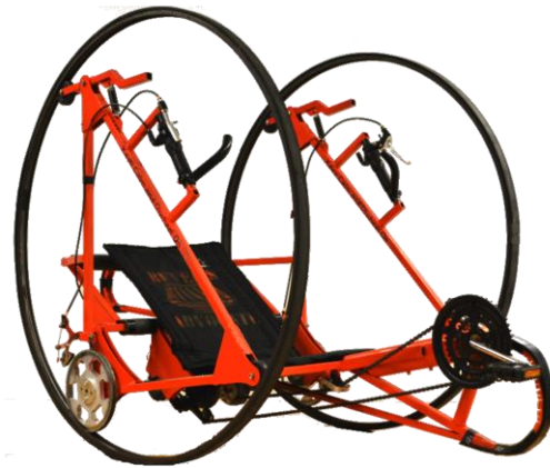
Figure 1: From concept to final fabrication, on the left is our fully rendered SolidWorks model, and on the right is the manufactured DiWheel.
