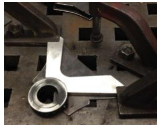
Jig for welding the shaft collar gusset assemblies
