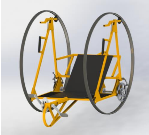
Figure 1: From concept to final fabrication, on the left is our fully rendered SolidWorks model, and on the right is the manufactured DiWheel.
