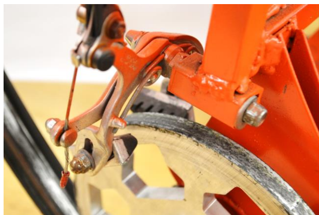
Brake mounted to the corner of the frame and positioned on the rim of the drive wheel.
