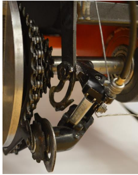
Cable Used to Pull the Derailleur into Better Tension with the Chain.
